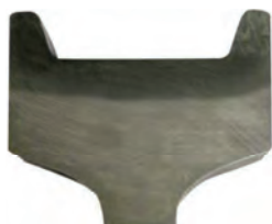
Deep Hardened™ Wheel Section (Based on a 27" Wheel Sample)
