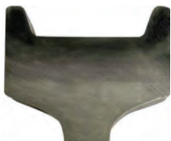
Rim Toughened Wheel Section (Based on a 27" Wheel Sample)
